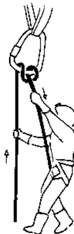
Figs 11 & 12 Lifeline controllers: friction knots (Above) the Italian Hitch: an extremely useful knot for lifelining; (below) a simple two-handed operation will take in slack rope as the climber ascends.
